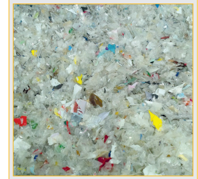
Output: Cleaned PET-tray flakes
