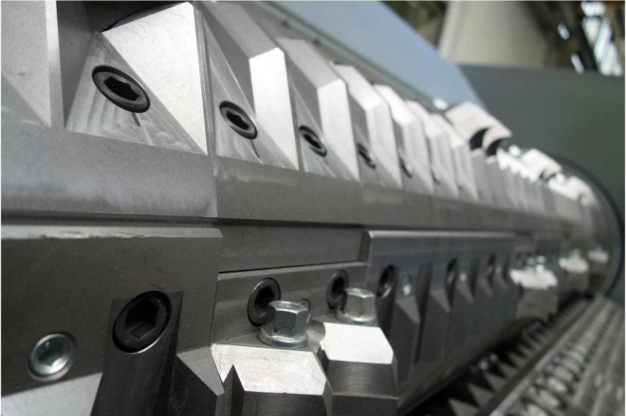
Figure 1: Rotor of a single-shaft shredder 60/210 with bolted-on knife cassettes.
