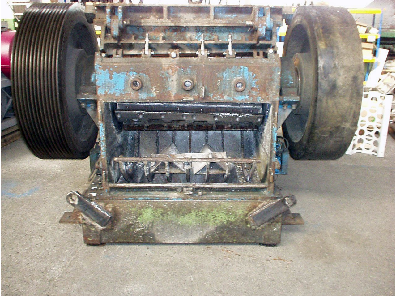
Figure 2a: A granulator SMS 80/120 before refurbishment.
