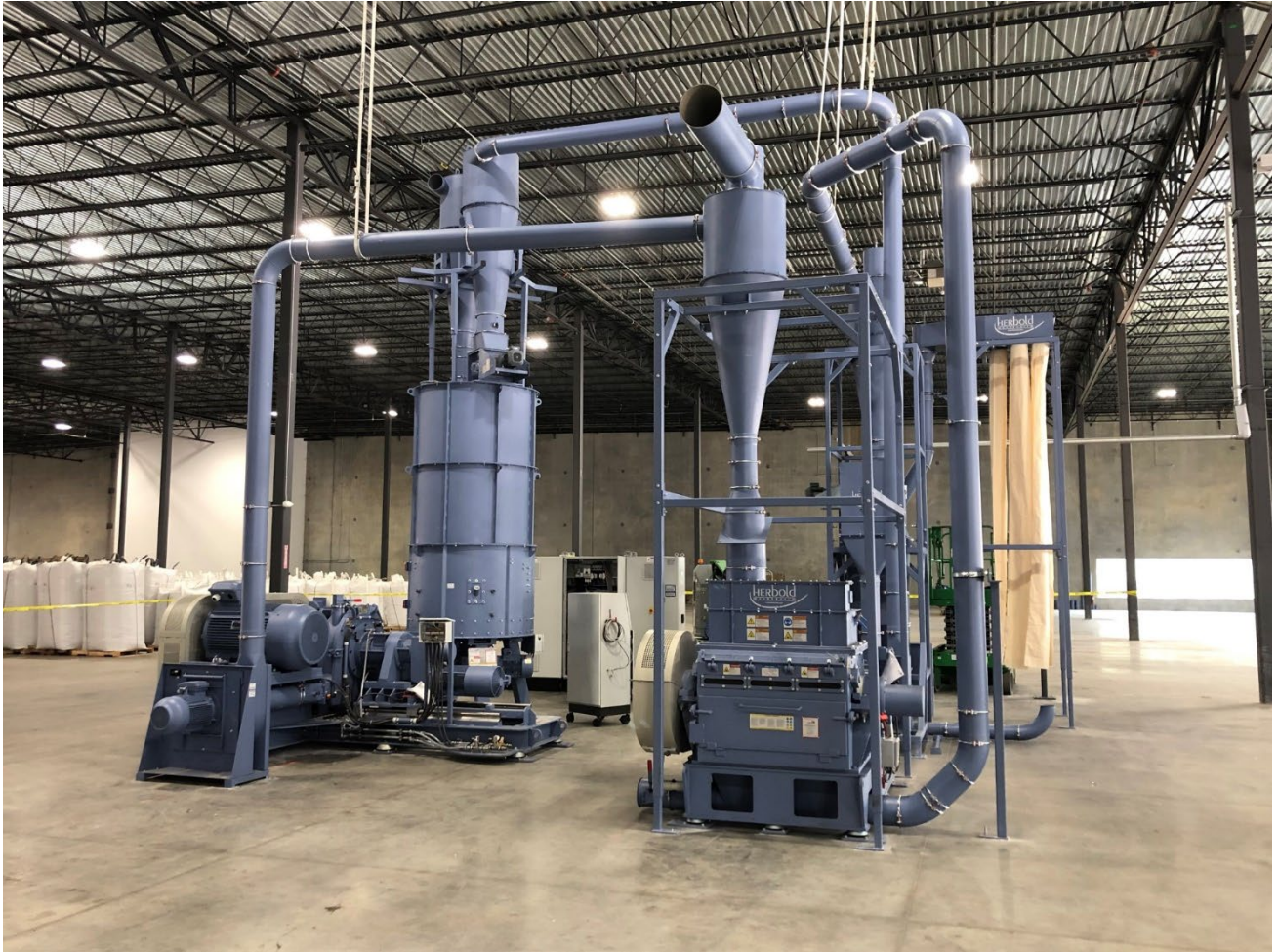
Figure 2: Agglomeration plant for fibers, fines, tapes, foams, films, powders or shavings.
